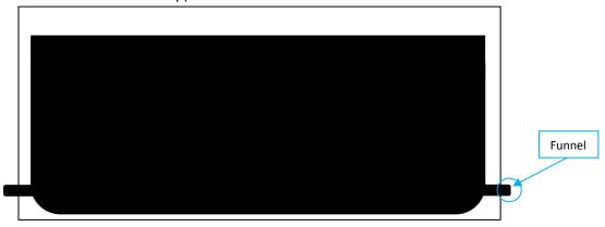
9. Make sure that all of the deflation zips are closed – one located on each side above the inflation funnel and one on the top of the screen in the middle.
